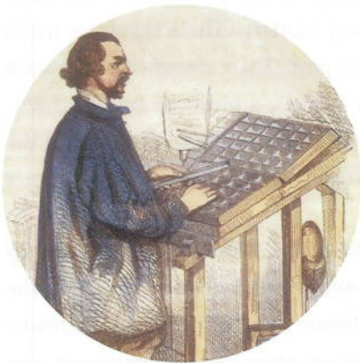
7.6 Typesetter at his composing stand of upper and lower case cast-metal letters.
